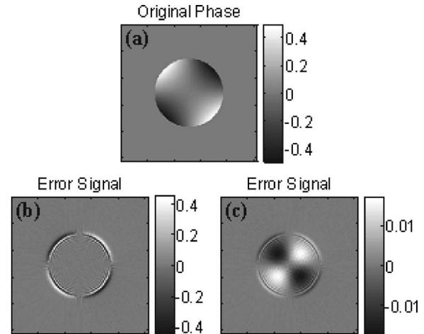
Fig. 1. (a) shows an astigmatic wavefront that is used to generate an error signal using phase diversity based on defocus. In (b) the error signal generated from a uniformly illuminated (i.e., hard-edged) pupil is shown. Note that the error signal is confined to the edge. For a soft-edged pupil (in this case a Gaussian profile with 10% drop in flux from center to rim) the error signal shown in (c) is uniformly distributed but of lower amplitude.
